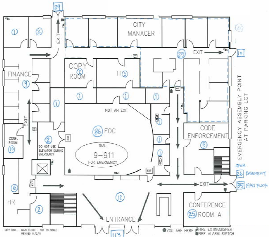
Exhibit 4C First Floor Occupancy Load and Exit Diagram
